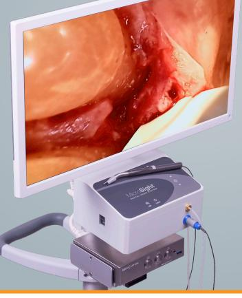
Q-Optics MicroSight<sup>®</sup> is an innovation in Video-Assisted Minimally Invasive Surgery technology. The MicroSight<sup>®</sup> videoscope utilizes patented Air Shield<sup>™</sup> Technology and integrated tissue retractor tip to achieve unprecedented visual access for minimally invasive procedures.
